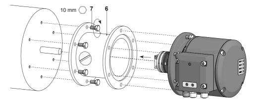
The encoder must be mounted with cable connection facing downward and not exposed to water.
